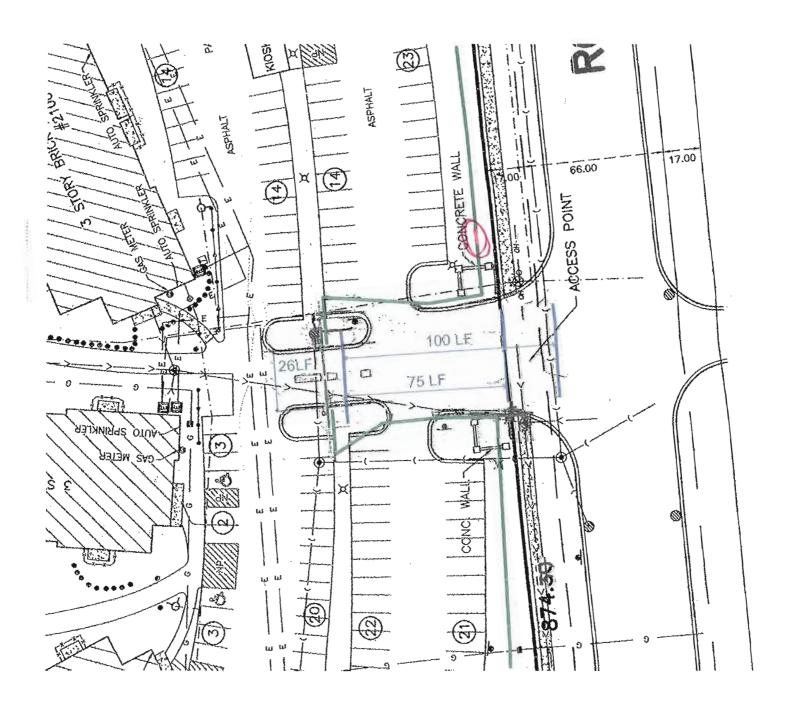
Proposal for Access 4 - Hassell Road and Georgetown Lane: Entrance way must be adjusted for 26' wide minimum openting. 2' wide curb islands installed by others as shown leaving opening for turn around.
