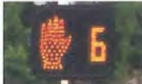
COUNTDOWN TIMER Indicates amount of time pedestrians have to cross. Helpful for people with disabilities and seniors. PHOTO: gothamist.com
