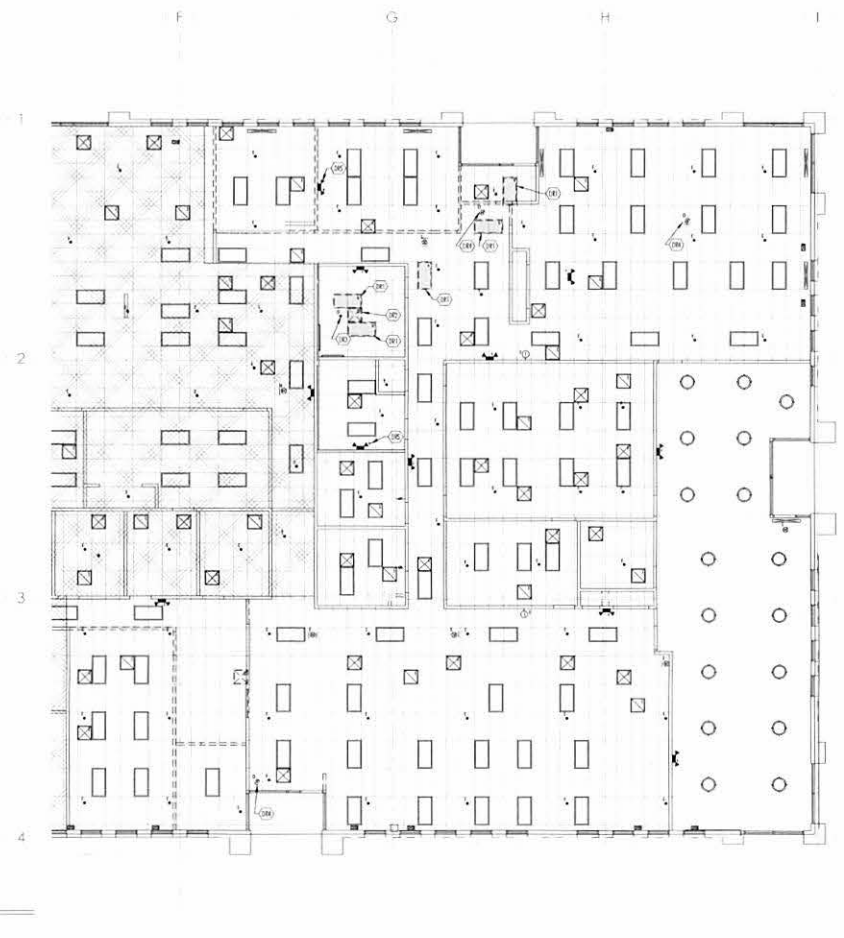
2 DEMO REFLECTED CEILING PLAN 1/8" = 1'-0"
