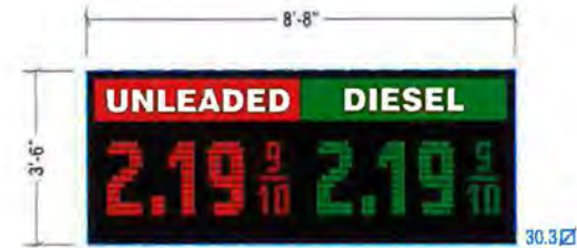
B ONE (1) SINGLE FACE, DOUBLE PRODUCT L.E.D. GAS PRICE DISPLAYS
