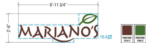
A1 A2 TWO(2) SETS OF FACE-LIT & HALO-LIT LETTERS & LOGO SCALE: 3/8" = 1'
