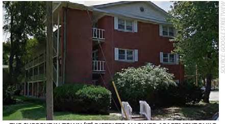
THE CURRENT IN-TOWN (IT) DISTRICTS ALLOWED APARTMENT BUILDINGS THAT LACKED A PRIMARY ENTRANCE, WITH TENANTS RELEGATED TO ACCESSING THEIR UNITS ON THE SIDE VIA EXTERIOR HALLWAYS. THIS LAYOUT ALSO HAD LITTLE RELATION TO THE STREET. THE NEW UN-1 AND UN-2 DISTRICTS WILL PROHIBIT THIS TYPE OF DESIGN.
