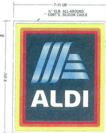
A Standard 'Flex-Face' Illum'd. Wall Sign TWO(2) req'd. scale: 3/8" = 1'-0"
