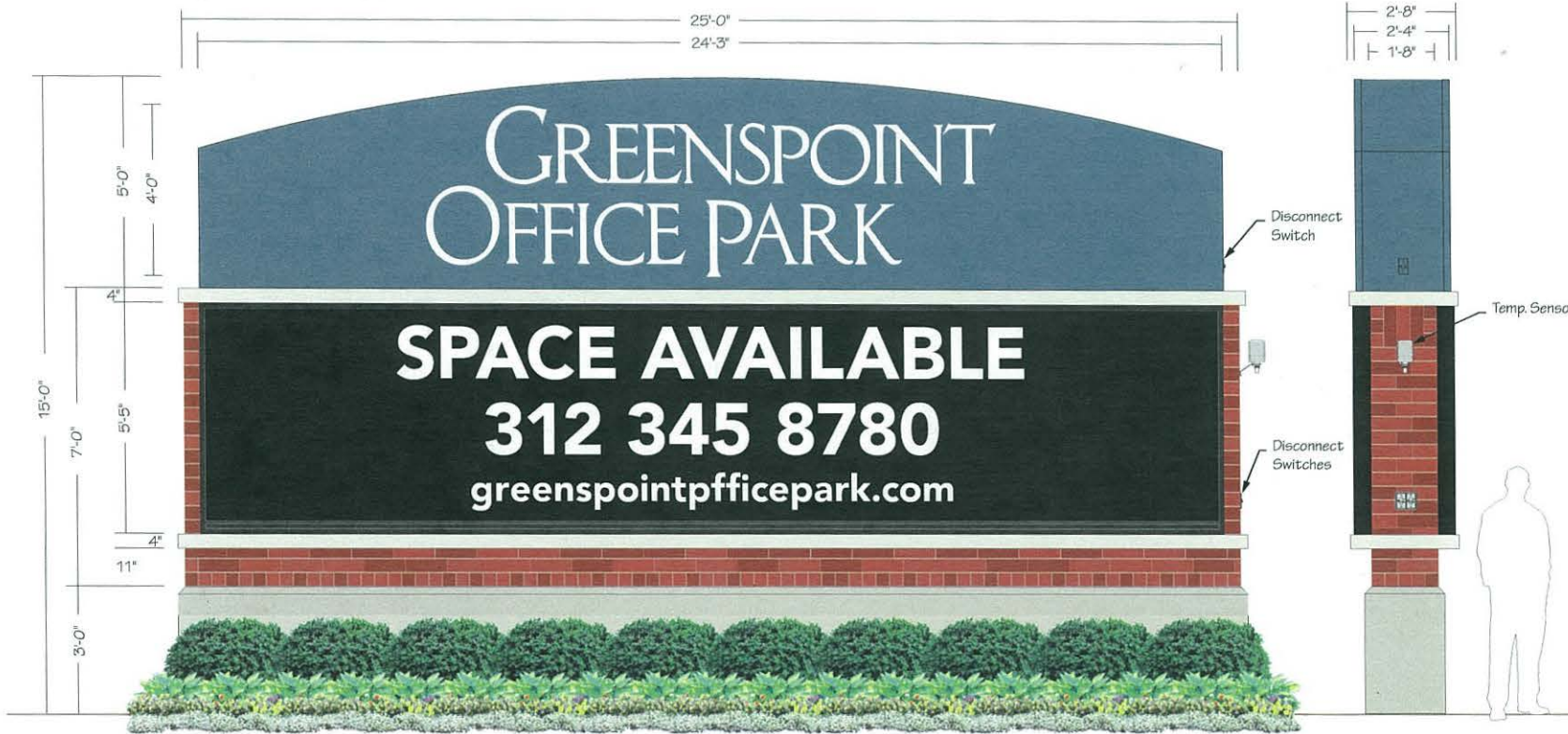
(1) 5'-0" x 24'-3" x 2'-8" Double Face Illuminated Monument Sign with EMC Units (15'-0" x 25'-0" x 2'-8" Overall)
