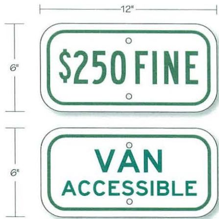
(2) 6" x 12" Single Face "FINE" & "VAN ACCESSIBLE" Panels
