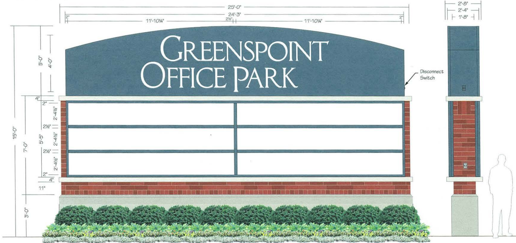
(1) 5'-0" x 24'-3" x 2'-8" Double Face Illuminated Monument Sign (15'-0" x 25'-0" x 2'-8" Overall)
